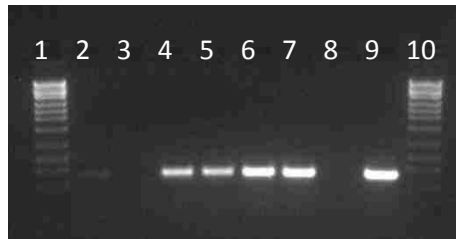
Figure 7. An additional test of the FISH to PCR assay detection limit. From left to right, the lanes are as follows: (1) 1kbp ladder, (2-6) FISH slides seeded with 1, 10, 100, 10^3 , and 10^4 oocyst(s), respectively, (7) DNA extraction positive control, (8) DNA extraction negative control, (9) primary PCR positive control, and (10) an additional 1kbp ladder (primary PCR negative control, secondary PCR positive control and secondary PCR negative control, all of which came out as
