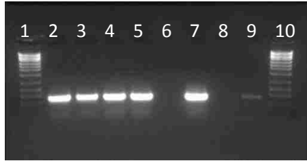
Figure 5. The FISH to PCR assay was first tested by seeding FISH slides with 10^4 oocysts. The secondary PCR products are shown after electrophoresis on a 1.4% agarose gel stained with ethidium bromide after 60 minutes. From left to right, the lanes are as follows: (1) 1kbp ladder, (2-4) samples spiked with 10^4 , (5) DNA extraction positive control, (6) DNA extraction negative control, (7) primary PCR positive control, (8) primary PCR negative control, (9) secondary PCR positive control and (10) an additional 1kbp ladder (secondary PCR negative control, which came out as expected, is not shown).
